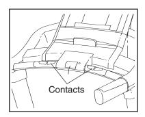
To measure your heart rate, stand on the foot rails and hold the metal contacts on the handrail—avoid moving your hands. Hold the contacts for approximately ten seconds. When your pulse is detected, your heart rate will be shown. For the most accurate heart rate reading, continue to hold the contacts for about 15 seconds.
